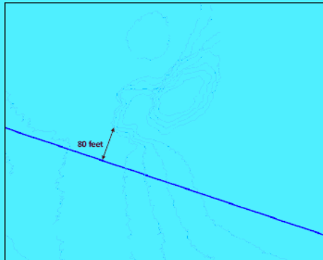
Figure 16 - Cable Route Separation from Rock Feature
